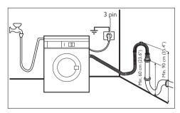
The drain hose may be extended to a maximum of 4 metres. An additional drain hose and joining piece is available from your
